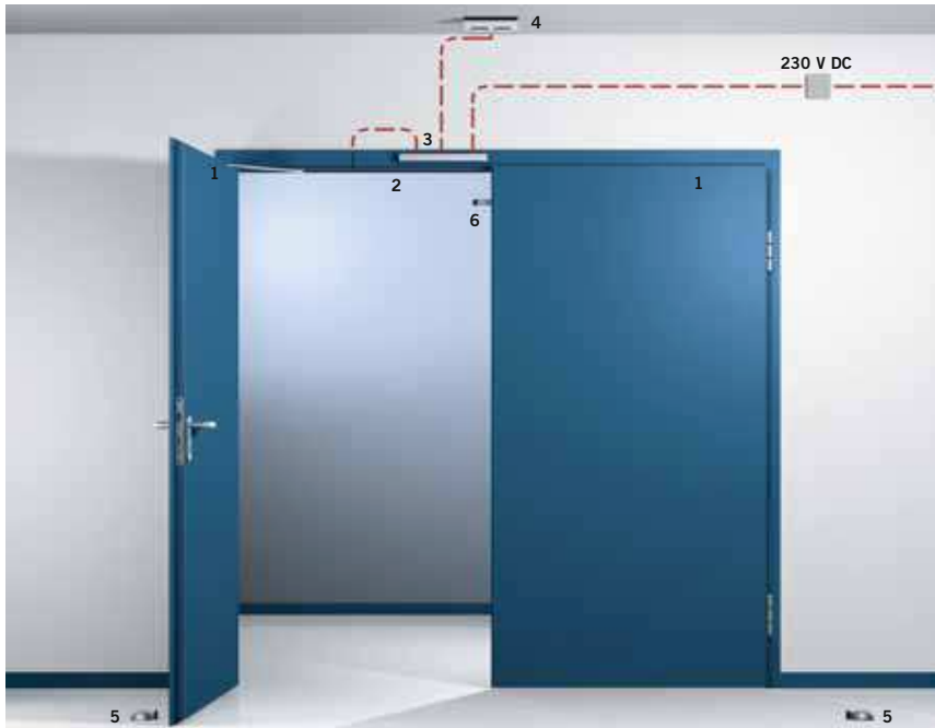
Application example: Hold-open system on a double door, comprising: Two door closers type DORMA ITS 96 (1); active and inactive slide channel DORMA G 96 G-SR-EMF (2) with push-rod clamping system; Contur design RMZ lintel-mounted smoke detector (3), and one DORMA RM ceiling-mounted smoke detector in the Contur design (4) on either side of the door; two door stops type OGRO TZ 5000 (5); carry bar MK 397 (6)
